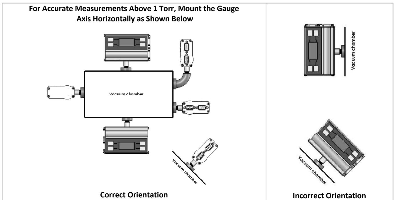
Mount the CVM201 with port down, if possible, to help minimize the effect of any particles or condensation from collecting in the gauge.
