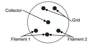
Base View BA601/BA602 EB degas - dual filament I<sup>2</sup>R degas - dual filament
